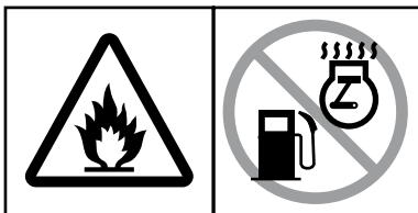
Petrol is highly flammable. Turn off the engine and allow time to cool before refuelling.
